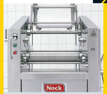
Quick and easy to clean: NOCK fish skinning machine after removing conveyors, pressure roller and blade holder
