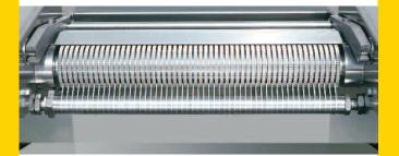
The automatic and the open top NOCK Cortex fish skinning machines are equipped with a **transport roller with grooves** (tooth roller). A **scraper comb** cuts in the grooves of the tooth roller and keeps it clean during operation.
