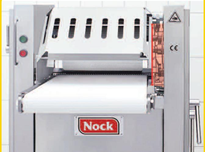
All machine parts which could obstruct the flow of the product, e.g. the mountings and handles of the blade holder, the mountings of the pressure device and of the conveyor belts, are located outside the tunnel-like safety cover.
