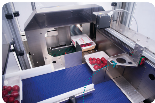
A Servo infeed pusher places the product in the banding arch
